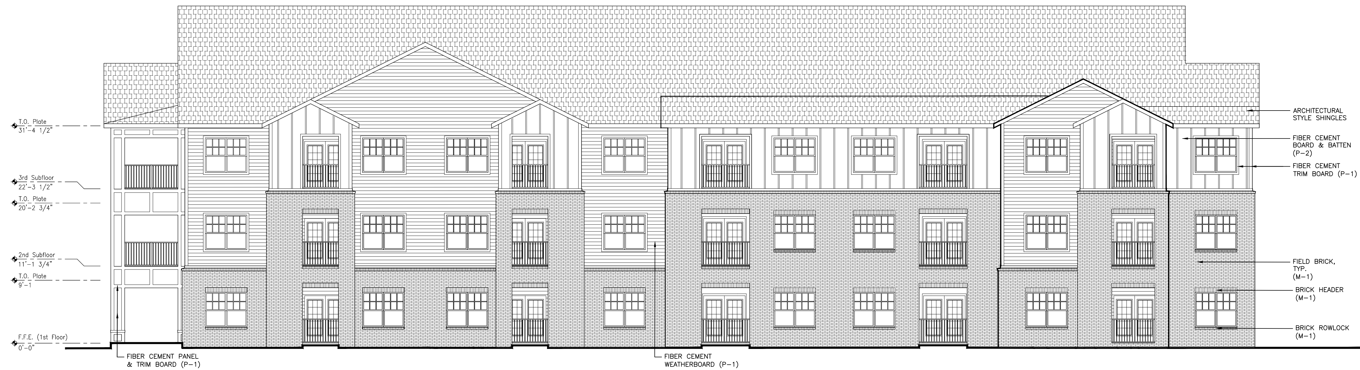
01 ELEVATIONS: Building Type I - Front/Rear 1/8" = 1'-0"
