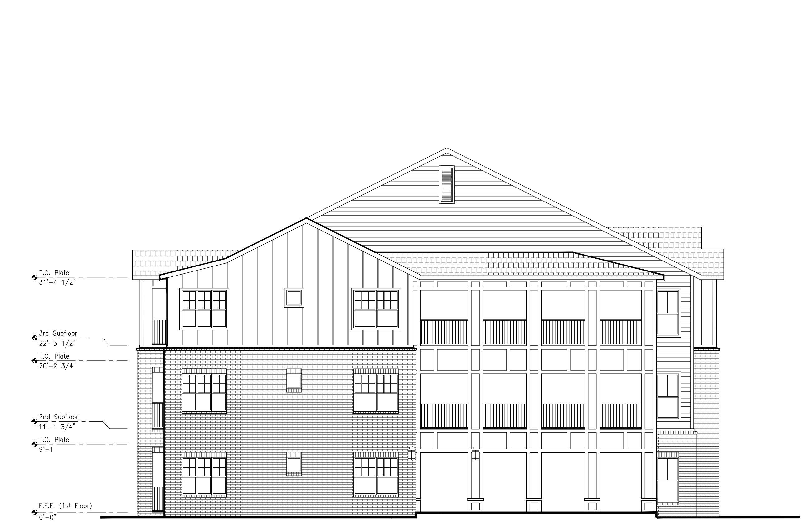
02 ELEVATIONS: Building Type II - Right 1/8" = 1'-0"
