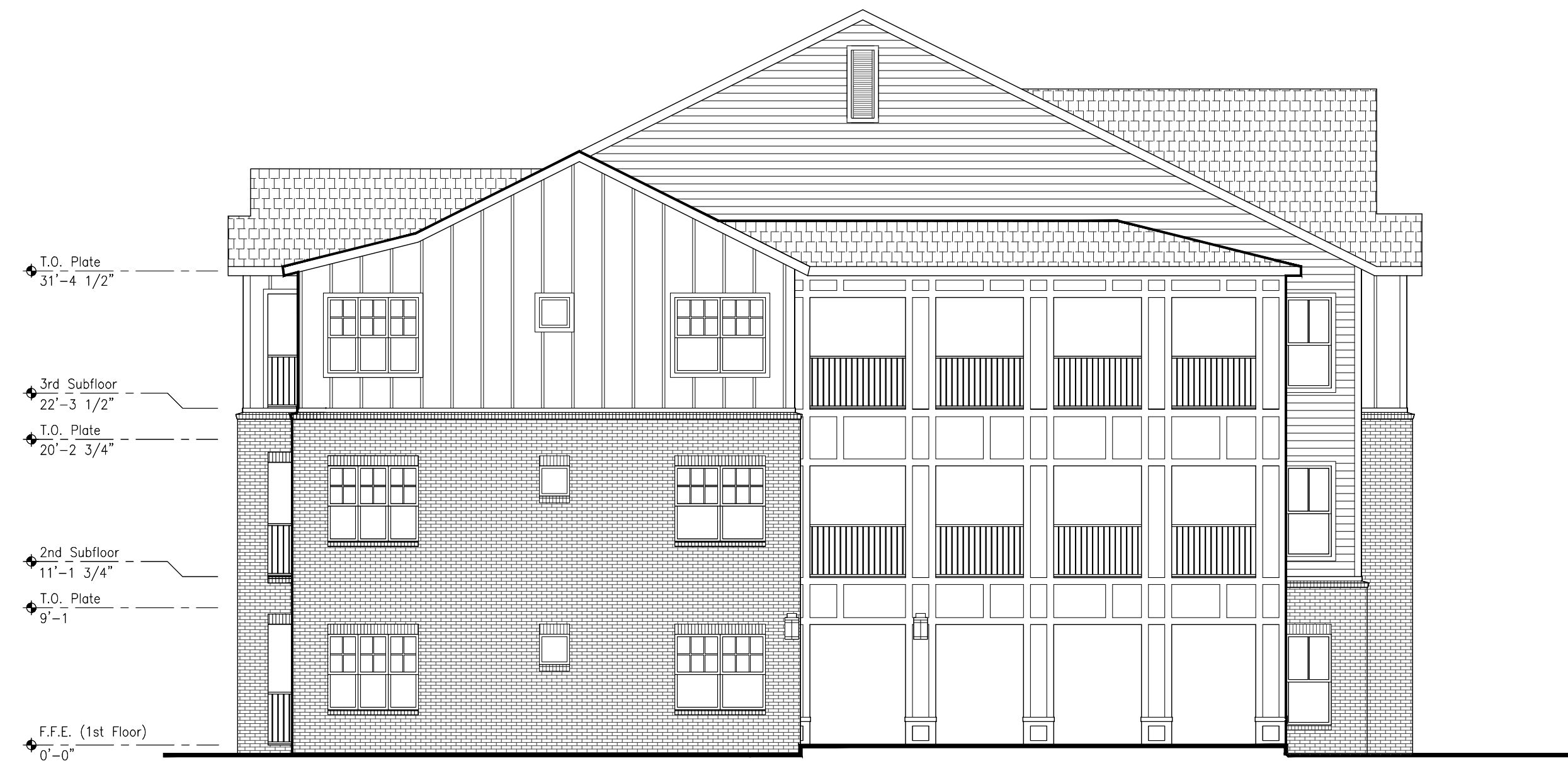
02 ELEVATIONS: Building Type I - Right/Left 1/8" = 1'-0"
